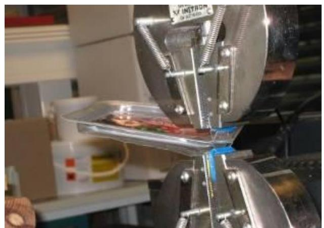
Figure 2 Mechanical measurement of the pulling force needed to open a cold cuts tray with flexible top foil and easy-peel (separation of top and bottom film).
