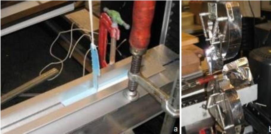
**Figure 2 Mechanical measurement of the pulling force of a) tear-strip in cardboard box (1. step) and b) ripping strength for the foil bag (2. step)-**
