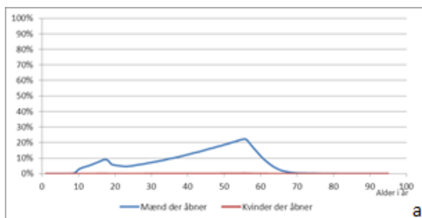
Figure 4 Share of men and women who are able to open a bag requiring a bag requiring a) 61N to open and b) 30N to open with a maximal gripping surface, in other words the "flap" being more than 2cm long (Model based on data from DTI, UK 2002).
