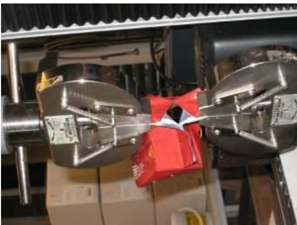
Figure 2 Mechanical measurement of the pulling strength when separating the wings of the foil bag.
