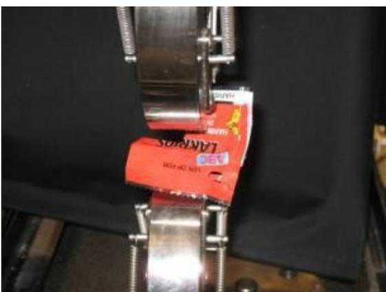
Figure 2 Mechanical measurement of ripping force needed for the candy bag with pre-cut.
