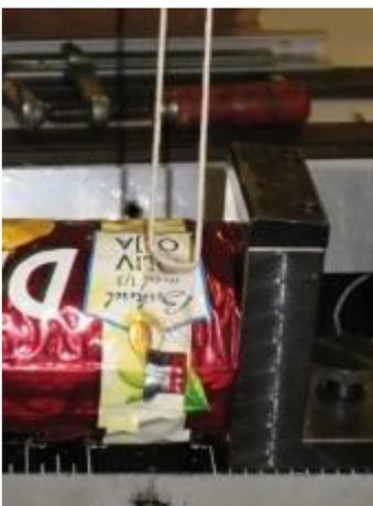
Figure 2 Mechanical measurement of the pulling strength needed for the tear-strip in the foil roll.
